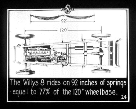
FOUR hydraulic, double acting shock eliminators control every movement of the springs.
