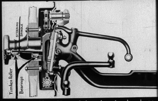
Timken roller thrust bearing in steering spindles makes steering an effortless operation.
