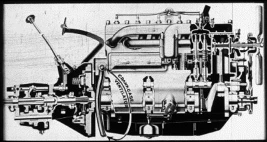
A crankcase ventilator reduces oil consumption and carries any fumes away from the interior of the car.
