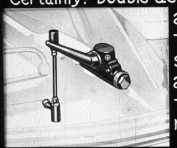
absorb the shocks and check the recoil.
