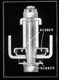
Rubber vibration absorbers at all four motor supports provide a maximum smoothness.
