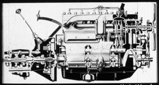
Note that oil passages are all drilled in the solid crankcase casting and crankshaft no leakage, no failures.
