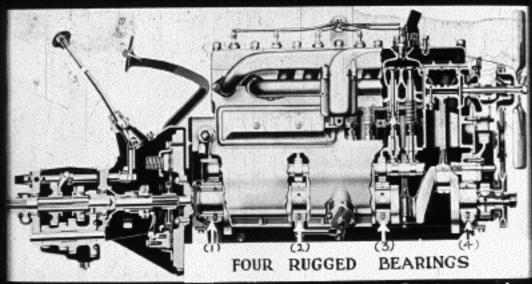
Counterbalanced Crankshaft has 4 Main Bearings\_ standard practice with cars costing twice as much!
