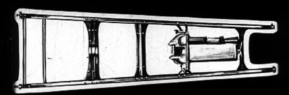
Frame is 5% inches deep and has SIX heavy cross members riveted to both top and bottom flanges.
