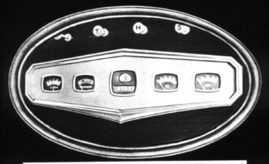
Four convenient buttons over the artistically grouped indicators, operate the choke, throttle, manual heat control and spark. Indirectly illuminated are the ammeter, heat indicator, speedometer, oil and gasoline gauges.
