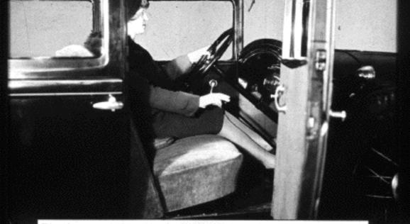
The longer shifting lever permits changing of gears without disturbance from a comfortable driving position and by the slightest wrist movement. The foot controls are within easy reach, yet not uncomfortably close.
