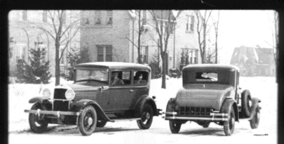
Notice how the proper placing of the slender center window pillars has removed them from the view of the driver. The shallow rear quarter permits clear vision of rear seat occupants and the narrow front pillars add safety to driving.
