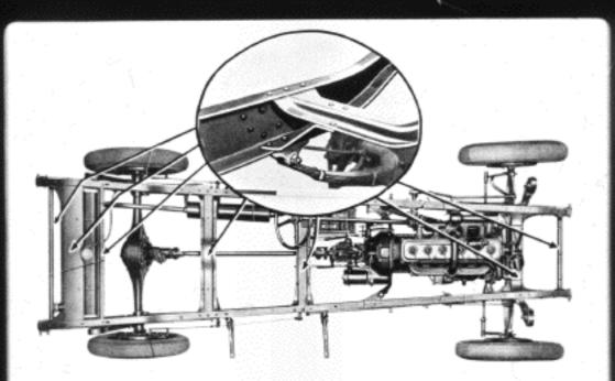
An advanced method of sturdy construction is introduced in this rugged frame. Note the number of cross members and the "dual anchored" principle which gives additional strength to the car's foundation.
