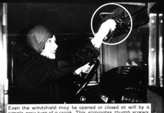
simple easy turn of a crank. This eliminates thumb screws, brackets, etc. and the task of loosening and tightening them. Instead of a "two-man" operation, adjusting the windshield is now a "one hand" operation.
