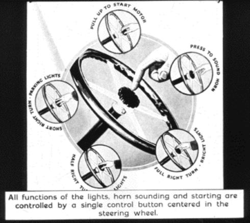
This is the most advanced convenience since the introduction of the self-starter. To start the engine, sound a warning and to place properly lighted highways at your instant command does not disturb you from a comfortable and safe driving position.
